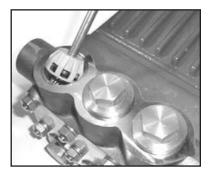
17. Next, place valve assemblies (46A) into manifold after first lubricating the o-ring (44A). Seat firmly into manifold.
